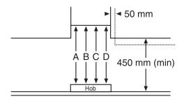
A: Built-in Electric Hob: 650mm minimum clearance
